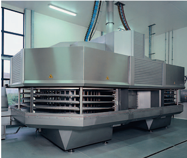
The SpiralOven in the open position providing excellent access
